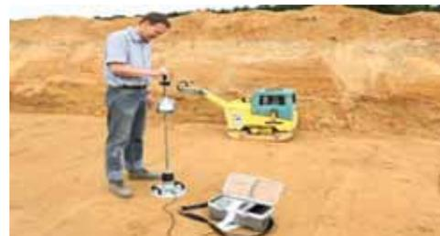
Image 6: dyn. Plate load test at ground level
