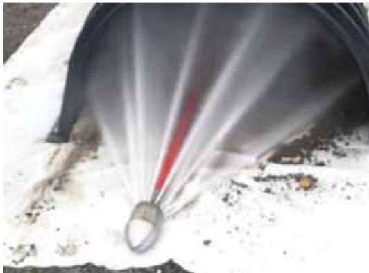
Image 3: Flushing nozzle with reverse conical jets
