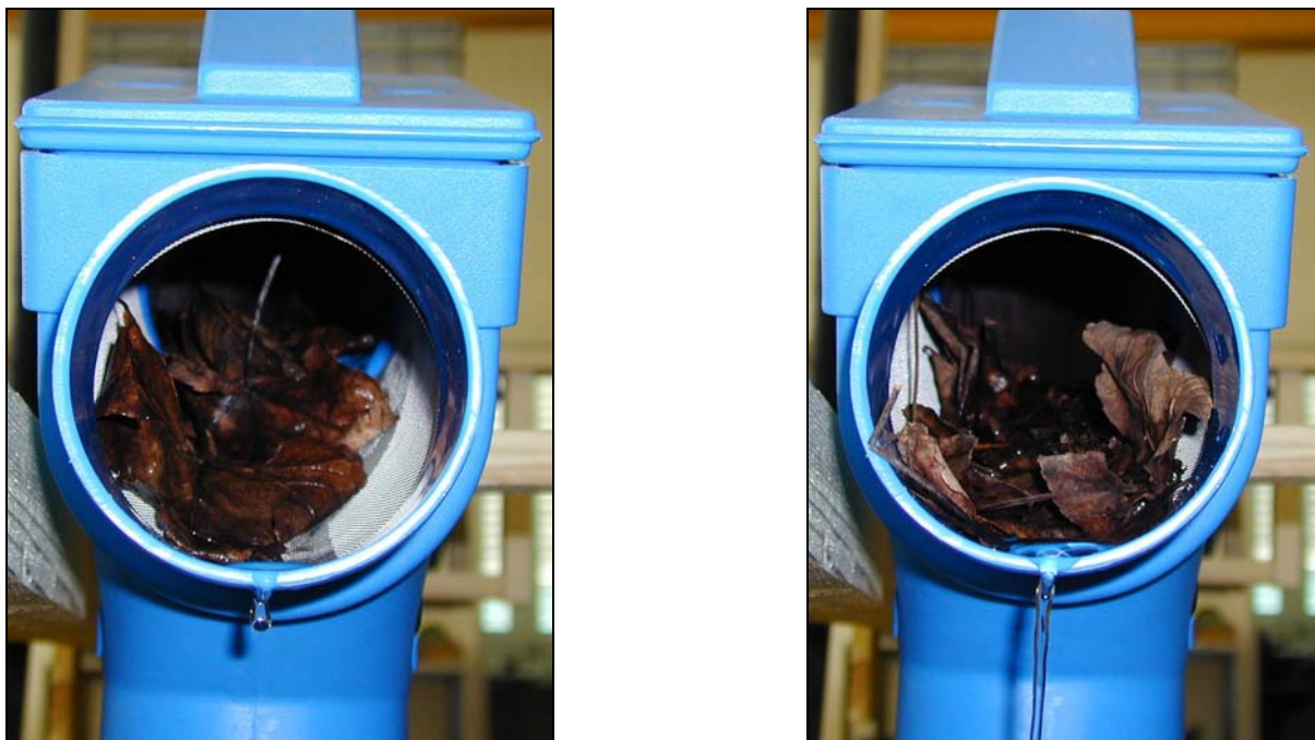
Figure 12: (left) 3P Cartridge filter PF with Q = 0.2 \text{ l/s} and dirt (Leaves)
