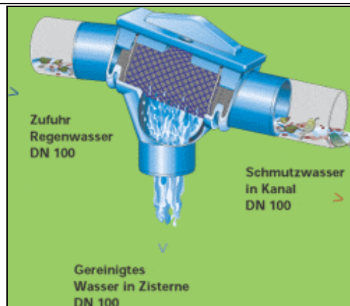
Figure 8: (right) Functioning principle of 3P cartridge filter PF
