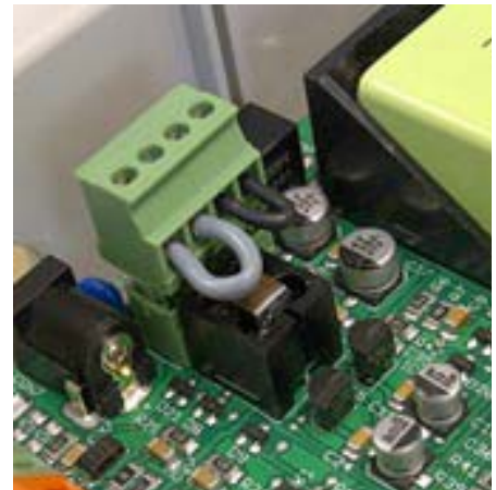
Fig.: cable bridge
