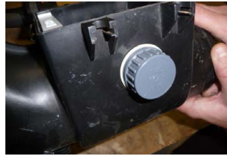
Fig. 3: Lateral sludge pump connection with stopper
