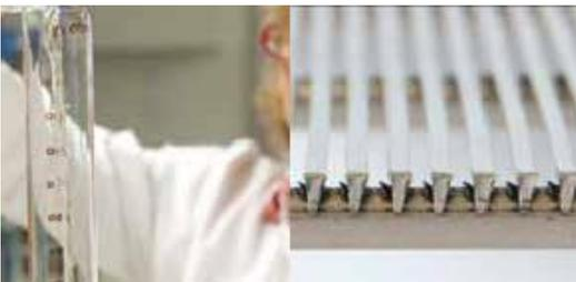
The sturdy wedge wire screen assures adequate water quality with no large debris being able to enter the cistern. The trapezoidal shape and diagonally set orientation prevents the dirt from settling and clogging it.
